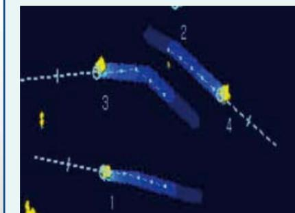
Clearly identifies moving targets from stationary targets. The display shows exact movement of other vessels like drawing tails. Even when your range is changed, a new trail appears past drawing tails. 3 types of shape is available.
